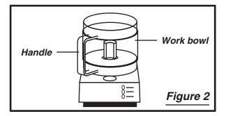
1. Put base on counter or table near an electrical outlet. Do not plug in until your Superstar food processor has been fully assembled. Pick up empty work bowl, holding it with handle toward you. Put bowl on base, fitting center tube over shaft on base and placing handle slightly to left of front center (7 o'clock).
