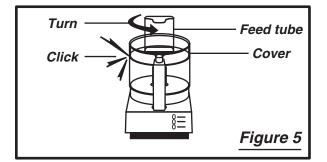
4. Put cover on bowl, with feed tube at front, slightly to left of front center.
