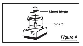
*3. Pick up metal blade by the center plastic part. Never touch metal cutting blades, which are razor sharp.*
