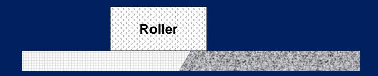
Make a roller pass in the vibratory mode overhanging 2 to 4-inches on the cold side.
