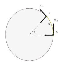
For the moment, assume the disk is rotating at a constant angular velocity  $\omega$ . Because of this, the length of the tangential velocity  $v^T$  vector is constant. The length of  $v^T$  is just the distance traveled S divided by the time of travel  $\triangle t$ , thus
