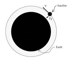
The radial force in this case is the force of gravity on the satellite by the Earth
