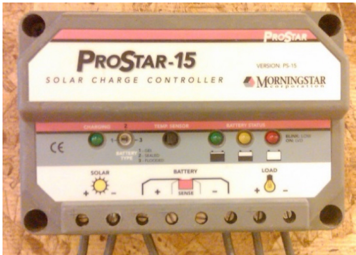
Figure 8. Examples of smaller-sized charger controllers. Example on top is rated for 10 amps, and example on bottom is rated for 15 amps.
