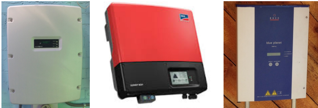
Figure 16. A string inverter connected in a system converts DC energy from the solar array to AC energy suitable for household power. Inverters come in various sizes based on total system power (wattage). A string inverter connected to a grid-direct system (sending energy to the local utility) detects utility-supplied energy blackouts and will automatically shut down for safety reasons. The inverter does not store energy, but converts it. If the array is not producing enough energy (lack of sunlight), the inverter will shut down.
