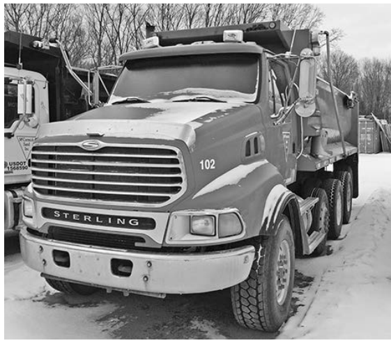
'02 Sterling LT9500 quad dump, Cat C15, 475 hp, 13 spd. manual trans., rock box, w/liftgate, set up to pull both tag & pup, lockers, eng. brake, 4.56 ratio, 535,000 miles, 18F, 44R, $70,000. (231) 206-6229
