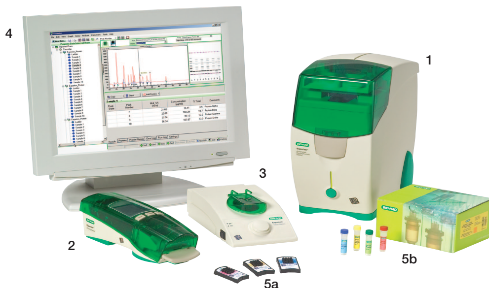
Fig. 1. The Experion system includes the following components: (1) automated electrophoresis station, (2) priming station (3) vortex station for nucleic acid analysis (4) system operation and data analysis software and (5) analysis kits (sold separately), which include the (a) chips and (b) reagents for protein, standard sensitivity RNA, high sensitivity RNA analysis, DNA 1K and 12K.
