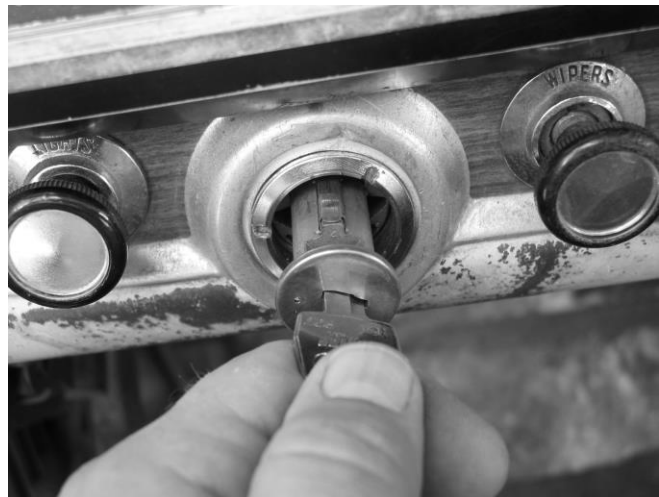
Step 4 – Pull the Lock Tumbler out of Switch
