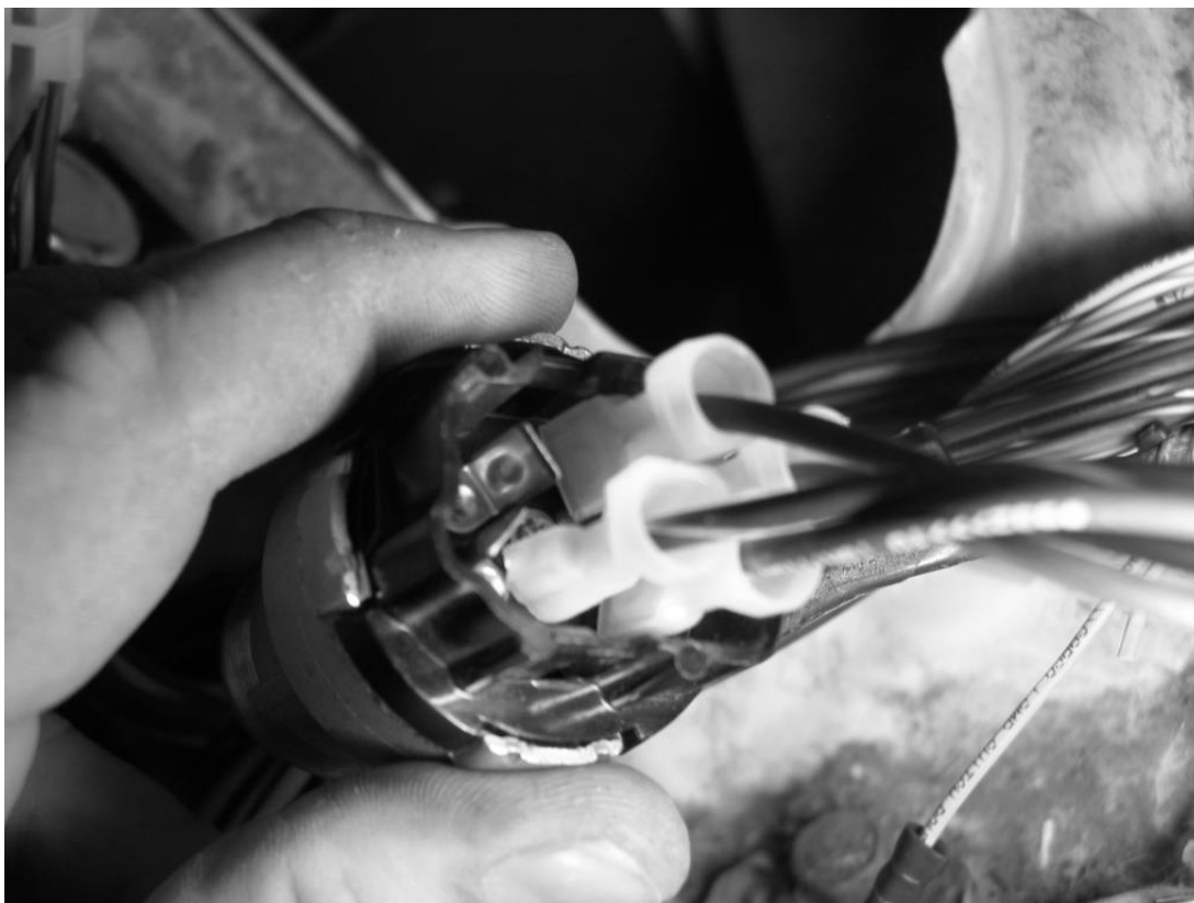
Figure 7-17 Ignition Switch Connections
