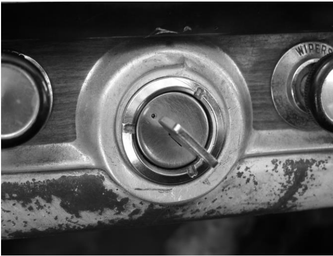
Step 1 – Turn Switch to ACC. POSITION
