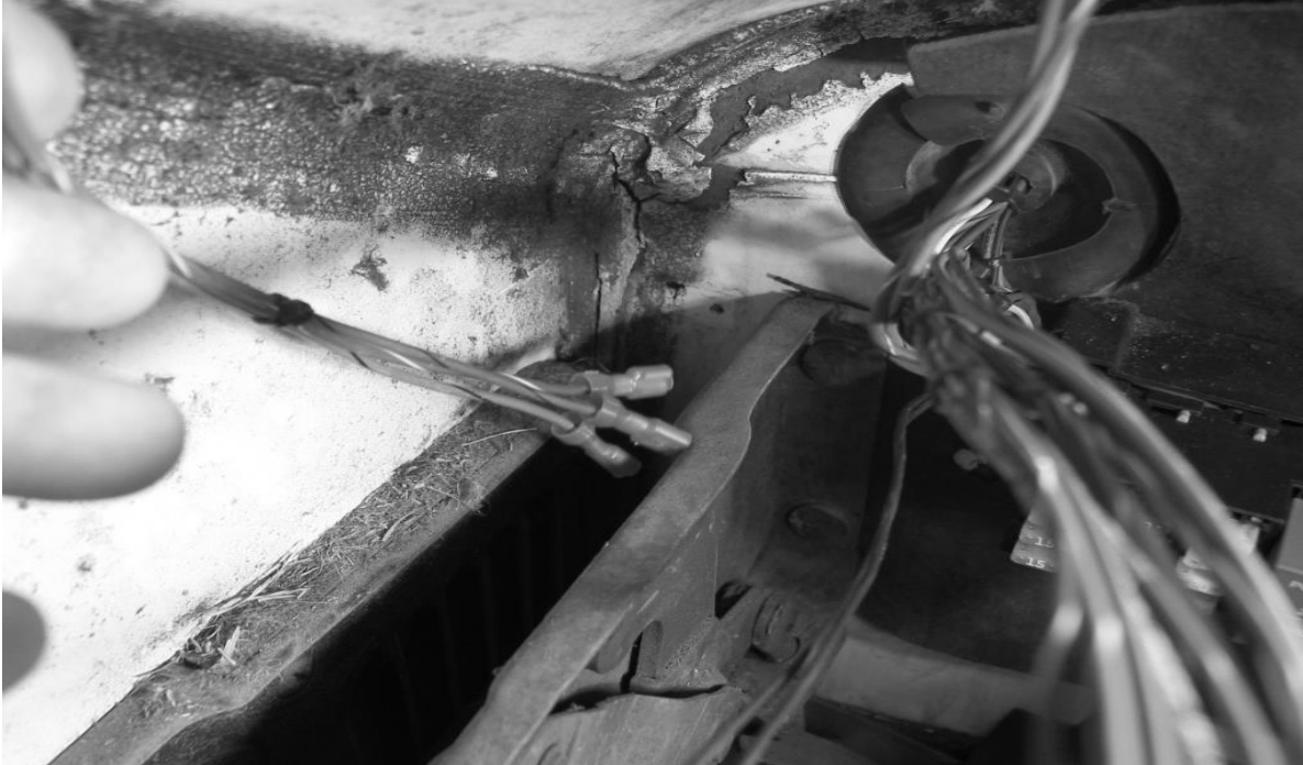
Figure 7-22 Routing the Dimmer Switch Wires
