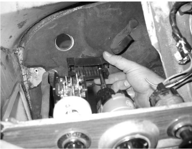
Figure 6-2 Fuse Block Base Position '67-'72
