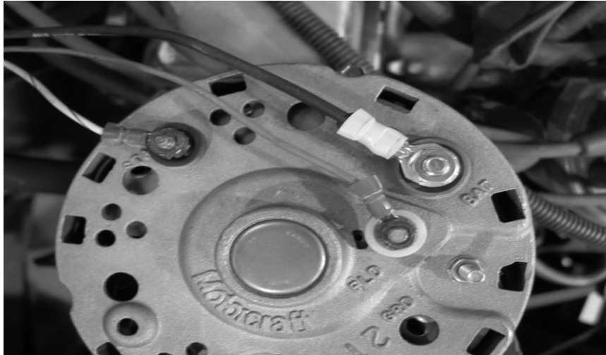
Figure 7-2 Alternator Connections '67-'77 Models
