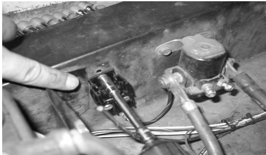
Figure 7-5 Installing the Maxi Fuse Holder '67-'72 Models
