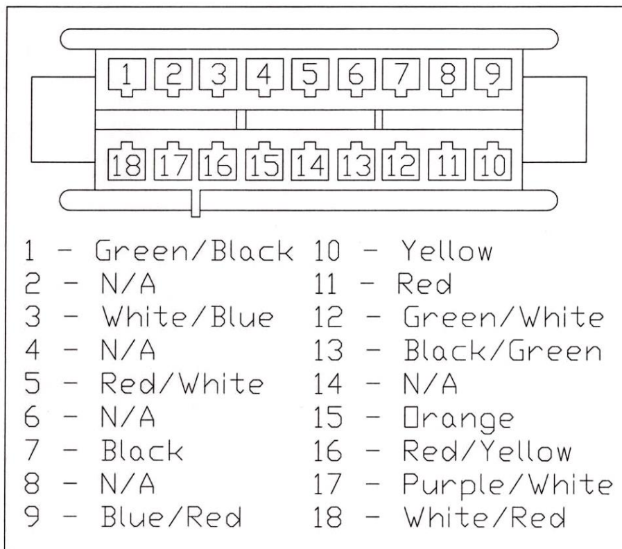
Figure 7-38 1973 - 1974 Cluster Pigtail Pinout
