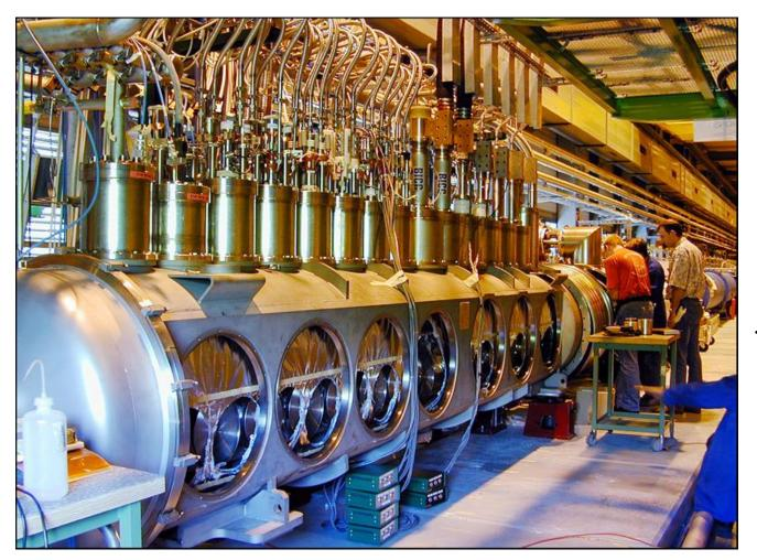
Many current leads and ports for access to make splice joints
