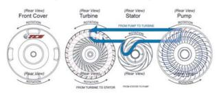
NOTE: Illustration shows all components as viewed from transmission end of torque converter
