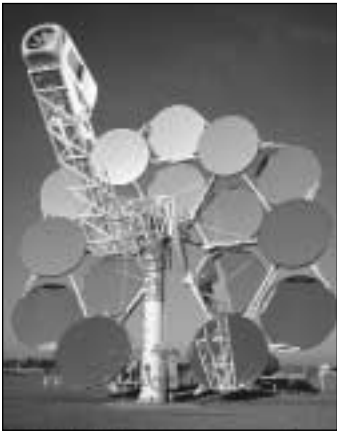
This dish/Stirling solar power system in Arizona is capable of producing 25 kW of electricity.
