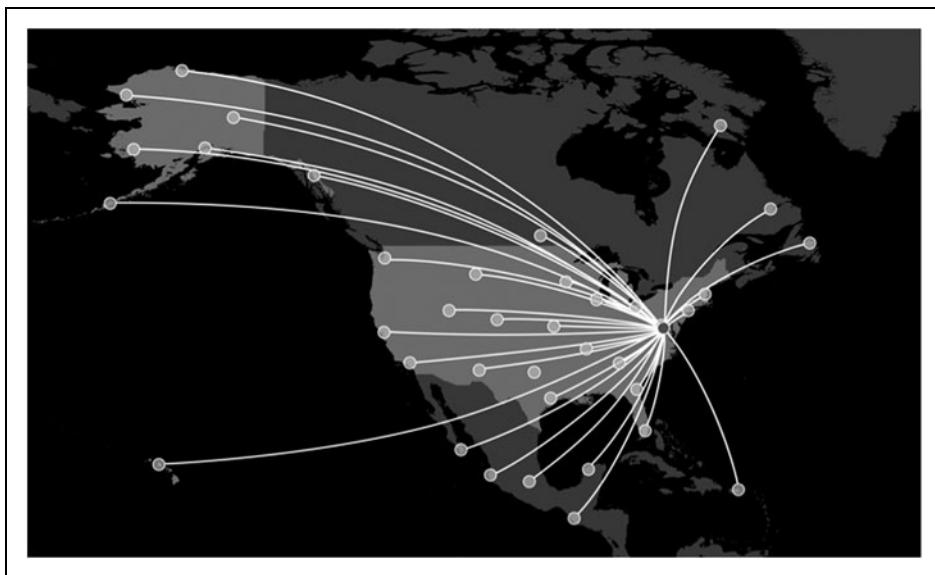
Fig. 15. WAAS showing the connections between the reference receivers and the WAAS master station on the East Coast. (Courtesy of BridgeNet International)
