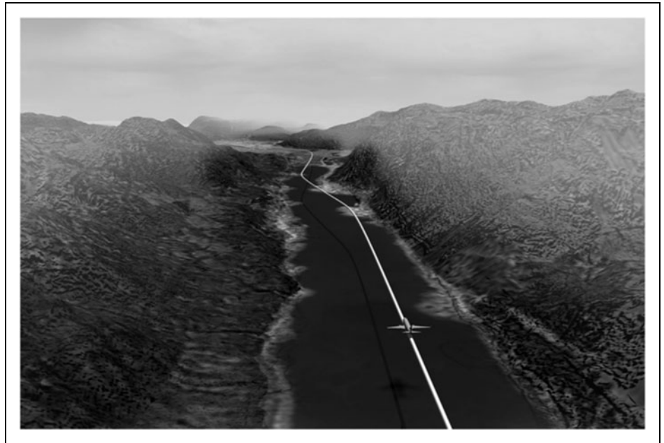
Fig. 5. Departures and arrivals from Juneau Airport (JNU) using the Gastineau Channel. The left turn at the far end of the channel, close to the airport, requires an area navigation (RNAV) capability. Such a path bend cannot be supported with a line-of-sight radio beam from the ground. (Courtesy of BridgeNet International)
