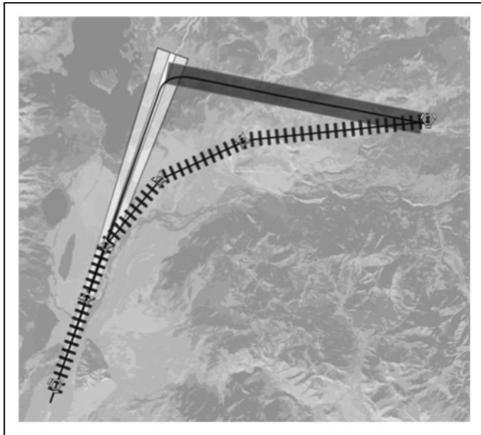
Fig. 6. Arrival to Jackson Hole (JAC) Airport using GPS-enabled RNAV. The RNAV path is curved and shorter, and avoids the main attractions of the Grand Teton National Park. (Courtesy of BridgeNet International)
