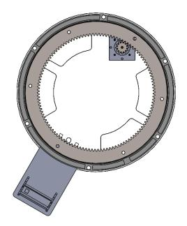
Figure 3: Top View of Turntable Assembly (without platform)
