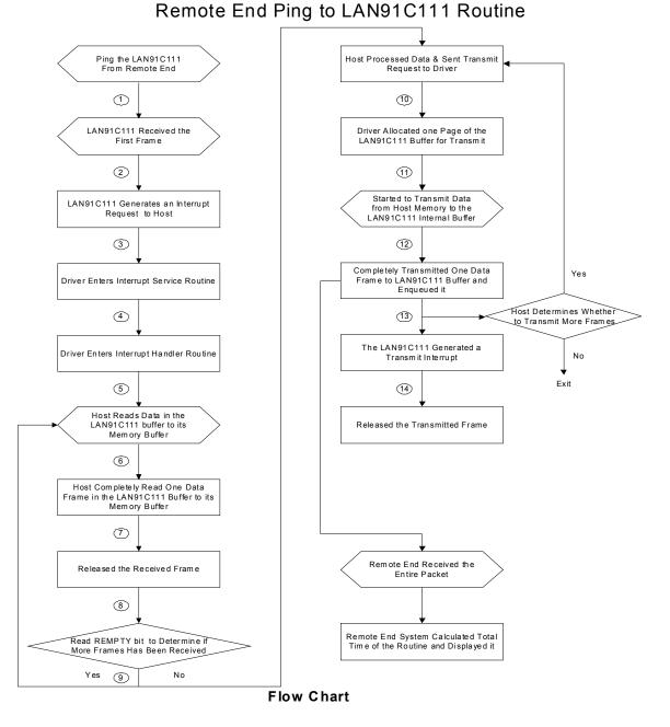
Figure 3.11 - Remote End Ping to LAN91C111 Routine
