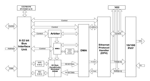
Figure 2.1 Detailed Internal Block Diagram
