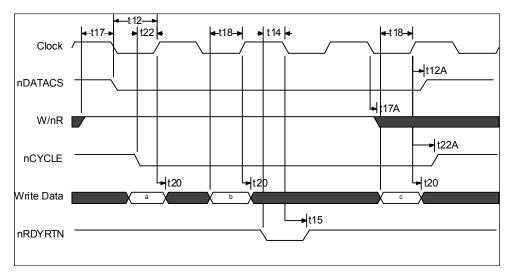
Figure 3.9 Burst Mode Write Operation
