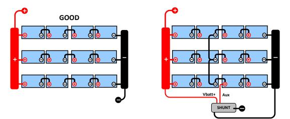
In an unmonitored battery bank the midpoints should not be interconnected, one bad battery bank can go unnoticed and could damage all other batteries.
