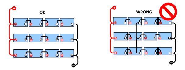
Due to the voltage drop over the positive and the negative cables the midpoint voltage are not identical.
