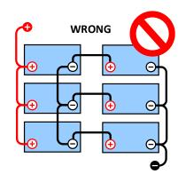
Due to the voltage drop over the positive and the negative cables the midpoint voltage are not identical.
