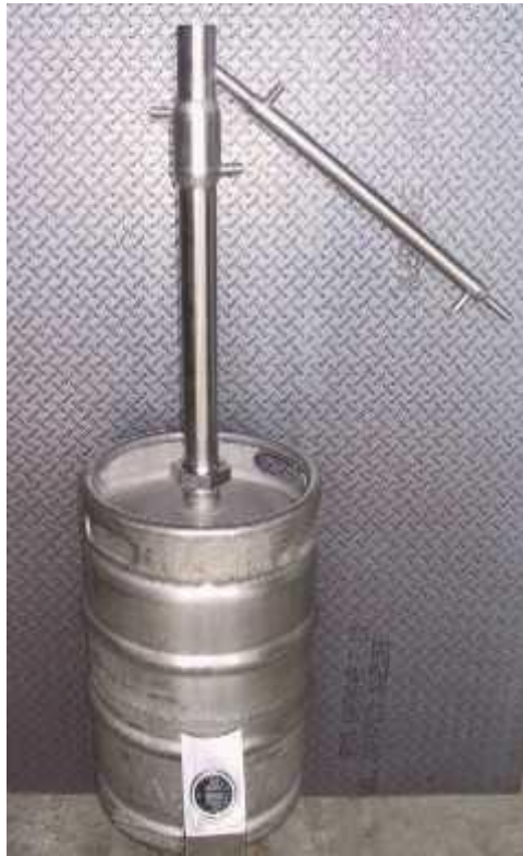
Stainless steel reflux still, fabricated in Australia , at Bosco Engineering P/L
