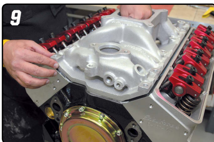
9 After adjusting the lifter pre-load to 3/4-turn, an Edelbrock RPM Air-Gap manifold is installed
