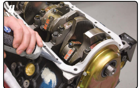
4 High quality parts like this one piece pan gasket ensure a leak-free engine
