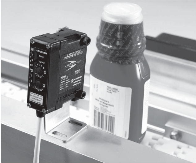
FIGURE 4 Advanced sensors working in pharmaceutical assembly systems help real-time operation control and quality assurance system to test every product. (This is often referred to as the zero-defect policy designed into a system.) The luminescence sensor illustrated will detect a wide variety of invisible targets. This STEALTH-UV sensor was designed to sense the presence of invisible fluorescent materials contained in or added to many products. Users can detect the most difficult targets, including clear tamper-proof seals, clear labels, and invisible registration marks. This unique sensor is also ideal for solving many of today's toughest problems in product orientation, inspection, and verification. (Courtesy of TRI-TRONICS Co., Inc., www.ttco.com .)
