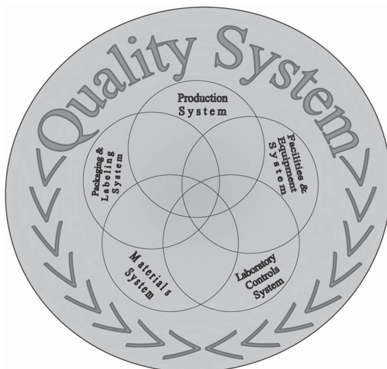
FIGURE 9 FDA's six-system inspection model.
