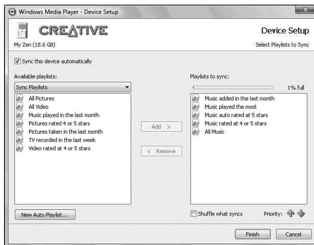
Figure 8.17 The Device Setup dialog box allows you to choose the playlists to sync and their priority.
