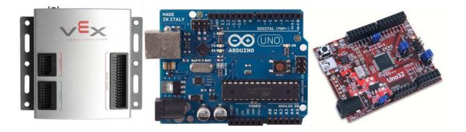
Figure 32: Vex PIC v0.5 Microcontroller, Arduino UNO, and chipKIT Uno32 (not to scale)
