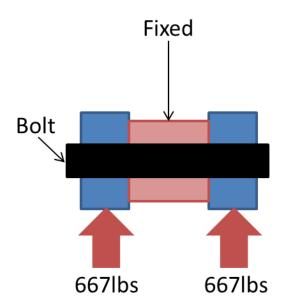
Figure 21: Diagram for pivot bolt in double shear
