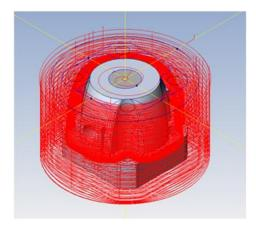
**Figure 42: Tool Path for Surface finishing**
