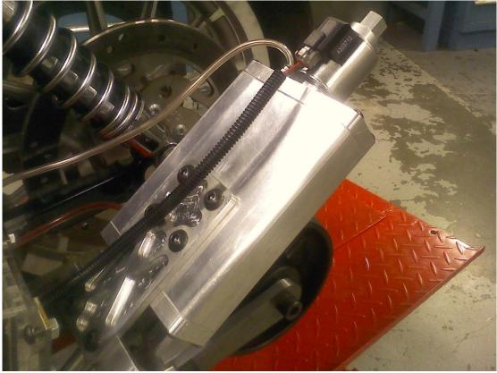
Figure 28: Installed Secondary Cylinder
