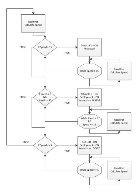
**Figure 31: Flow Chart of Test Program**
