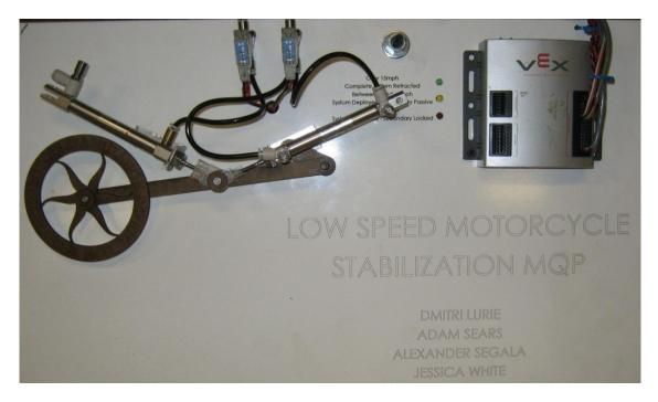
Figure 30: Proof of Concept Model Using VEX Components
