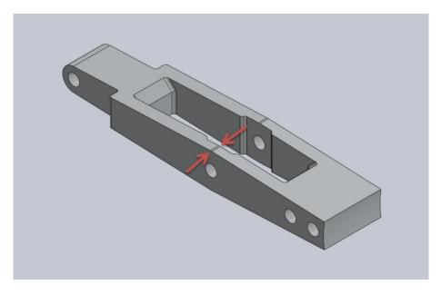
**Figure 19: Point of Highest Stress in the Lower Link**
