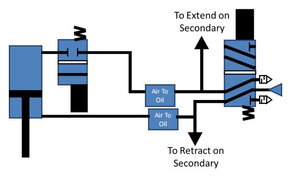
Figure 24: Deployment Cylinder Schematic
