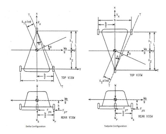
Figure 11: Free-body diagrams for Delta and Tadpole Configurations (*Three Wheeled Vehicle Dynamics*)
