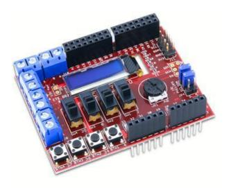
Figure 34: chipKIT Basic I/O Shield
