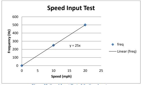
**Figure 35: Speed Input Test of the Speedometer**
