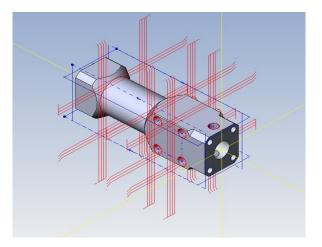
Figure 40: Esprit generated 4-axis tool paths
