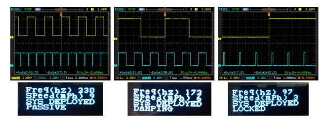
Figure 37: Oscilloscope Readings and Display for Different Conditions
