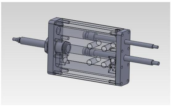
Figure 29: Internal Configuration of Secondary Cylinder
