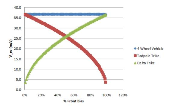
Figure 12: Rollover stability to Lateral Acceleration
