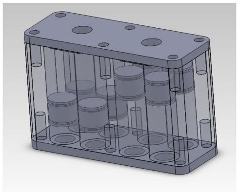
Figure 26: Solid Model of Air to Hydraulic Convertor
