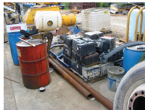
Waste materials are left exposed to the elements and stormwater runoff. Lack of secondary containment for the tank.
