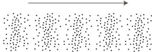
Vibrating air particles pass the energy of the vibrations away from the string in waves.
