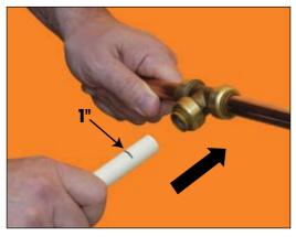
Ensure pipe is cut square and rough edges and debris are removed. Push pipe and fitting together to a 1" depth for permanent joints with Copper, CTS CPVC and PEX. Disconnect clip is available separately. Complete details at www.cashacme.com
