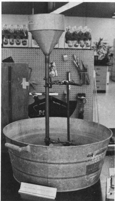
This apparatus found in the old Eaton Lab served to test abrasion effects on different products, measured by the impact of falling sand.
