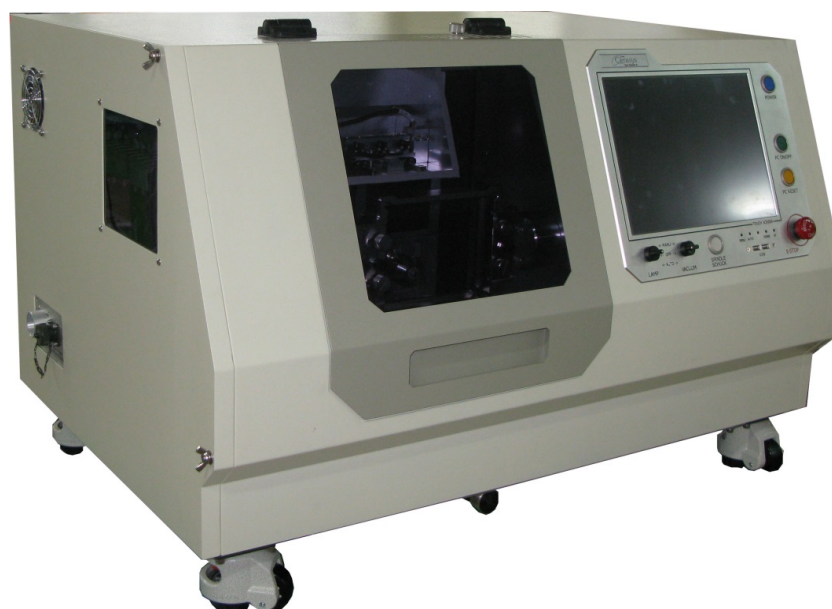
Figure 3. Dental CAD/CAM milling machine. Courtesy: Robots and design, Seongnam city, Gyunggi-do, Korea.
