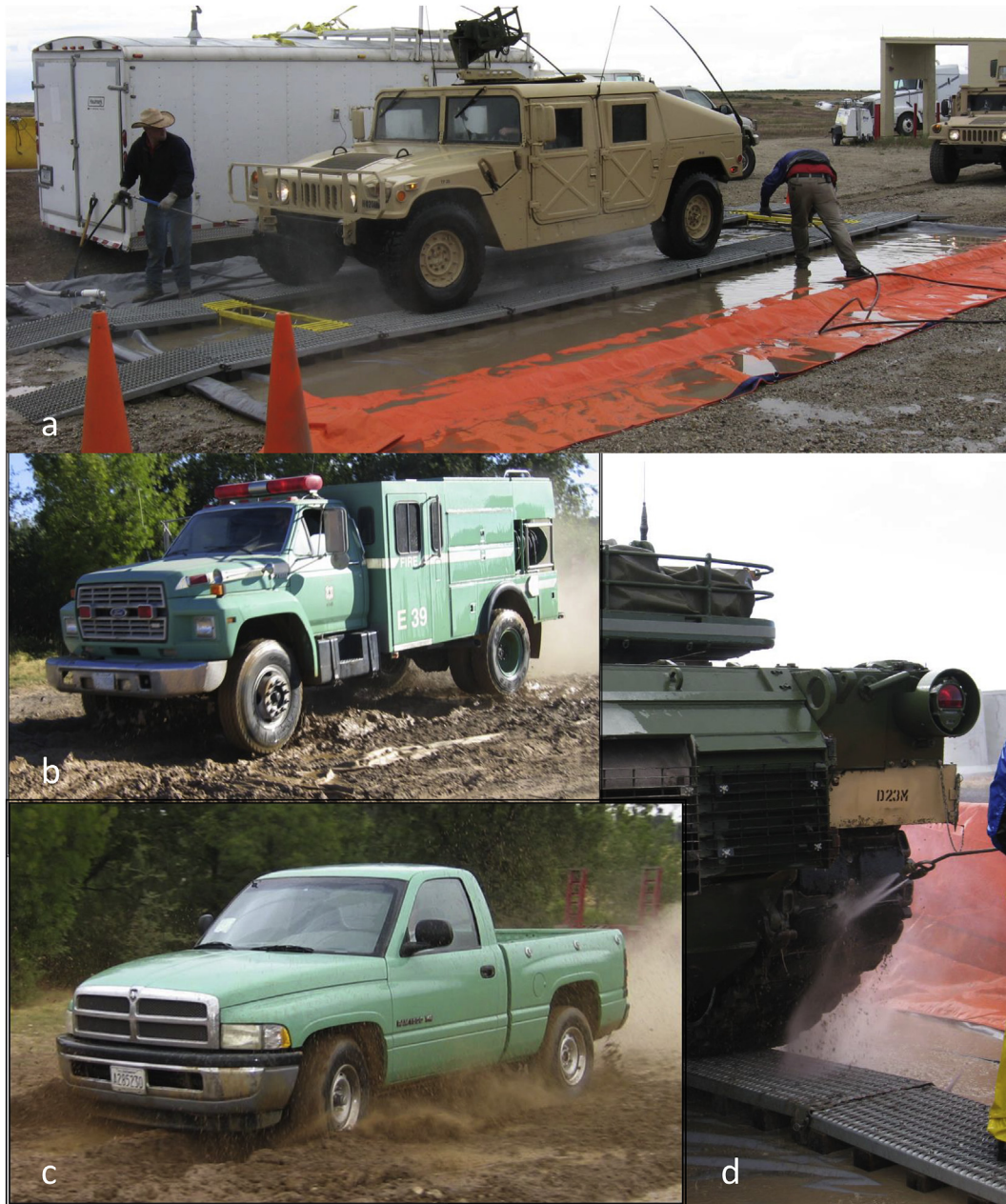
Fig. 1. The primary vehicle wash unit's (VWU) containment mats including raised edges, wheel racks, undercarriage washes and hand held wands are shown in a and d, and the artificially created mud bog used to evaluate VWU effectiveness is shown b and c. Vehicle types are as follows: 4WD (Humvee in a and truck in c), large 4WD in b, tracked - M1A1 tank in d.
