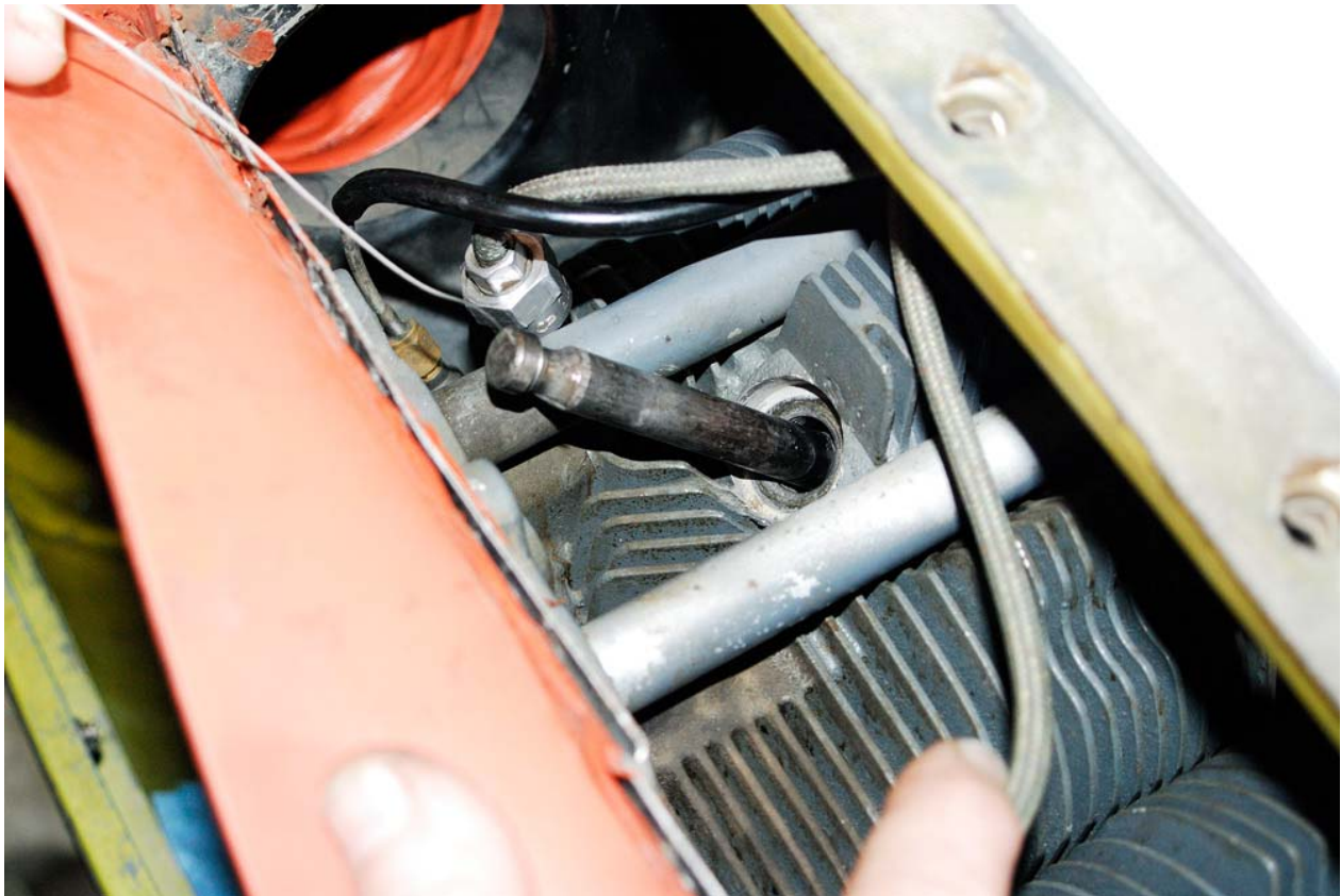
Valve stem in spark plug hole
