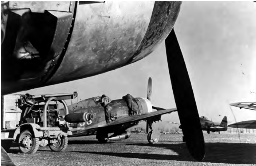
A crane is used to transfer bombs from storage to be mounted beneath the wing of a P-47 (top); and at a French railroad station, airmen load crated bombs onto trucks destined for Ninth Air Force airstrips (bottom).
