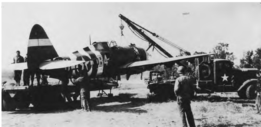
Mechanics hoist a severely damaged P-47 onto a trailer to be stripped of all usable parts (top); only a few miles behind enemy lines (right), these soldier-technicians are refueling, rearming, and checking planes for the next mission.
