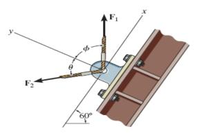
The parallelogram law of addition and triangular rule are shown in Figs. a and b, respectively.
