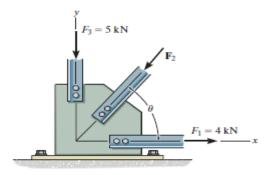
This problem can be solved by adding the forces successively, using the parallelogram law of addition, shown in Fig. a. Two triangular force diagrams, shown in Figs. b and c, can be derived from the parallelograms. For  $\mathbf{F}_{l}$  to be minimum, it must be perpendicular to the resultant force's line of action. Thus,
