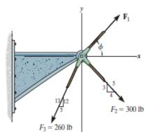
**Rectangular Components:** By referring to Fig. *a*, the *x* and *y* components of  $\mathbf{F}_1$ ,  $\mathbf{F}_2$ ,  $\mathbf{F}_3$ , and  $\mathbf{F}_R$  can be written as
