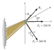
Rectangular Components: By referring to Fig. a, the x and y components of F1, F2, and F3 can be written as
