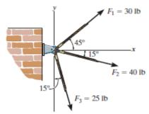
**Rectangular Components:** By referring to Fig. a, the x and y components of  $F_1$ ,  $F_2$ , and  $F_3$  can be written as
