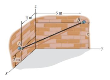
**Position Vector:** The coordinates for points A and B are A(3, 0, 2) m and B(0, 6, z) m, respectively. Thus,
