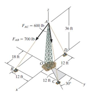
**2–121.** Determine the magnitude of the projected component of force  $\mathbf{F}_{AC}$  acting along the *z* axis.
