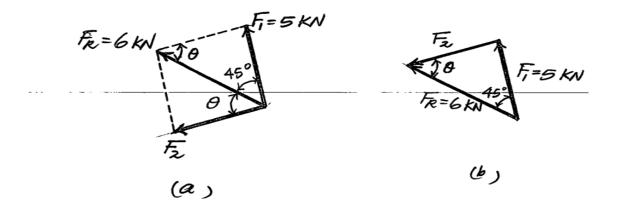
**2–24.** If the resultant force  $\mathbf{F}_{\mathbf{R}}$  is directed along a line measured 75° clockwise from the positive *x* axis and the magnitude of  $\mathbf{F}_2$  is to be a minimum, determine the magnitudes of  $\mathbf{F}_{\mathbf{R}}$  and  $\mathbf{F}_2$  and the angle  $\theta \leq 90^\circ$ .
