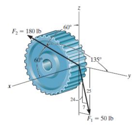
2–77. Determine the magnitude and coordinate direction angles of  $F_2$  so that the resultant of the two forces is zero.
