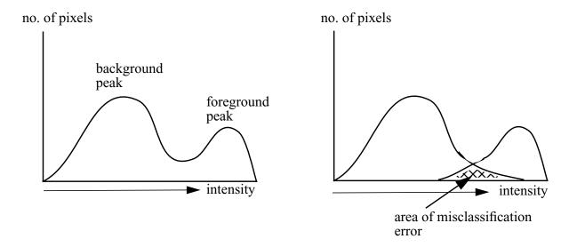
**Figure 2.** Illustration of misclassification error in thresholding. On left is intensity histogram showing foreground and background peaks. On right, the tails of the foreground and background populations have been extended to show the intensity overlap of the two populations. It is evident that this overlap makes it impossible to correctly classify all pixels by means of a single threshold. The minimum-error method of threshold selection minimizes the total misclassification error.
