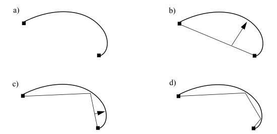
Figure 2. Illustration of the iterative endpoint algorithm. a) The original curve. b)
