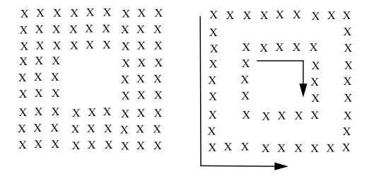
**Figure 1.** On the left is a region, where the ON-valued pixels are represented by "X"s. On the right is the contour of this region, where only the outer and inner boundaries remain ON. The arrows around the contour show the direction of coding.
