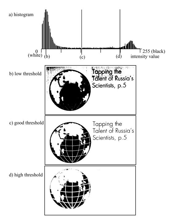
**Figure 1.** Image binarization. a) Histogram of original gray-scale image. Horizontal axis shows markings for threshold values of images below. The lower peak is for the white background pixels, and the upper peak is for the black foreground pixels. Image binarized with: (b) too low a threshold value, c) a good threshold value, and d) too high a threshold value.
