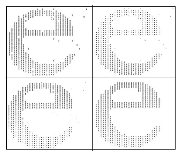
**Figure 3.** Results of kFill filter for salt-and-pepper noise reduction. The original noisy image is shown at the top left. The top right shows ON pixel removal, the bottom left shows OFF pixel filling, and the final image is shown in the bottom right.
