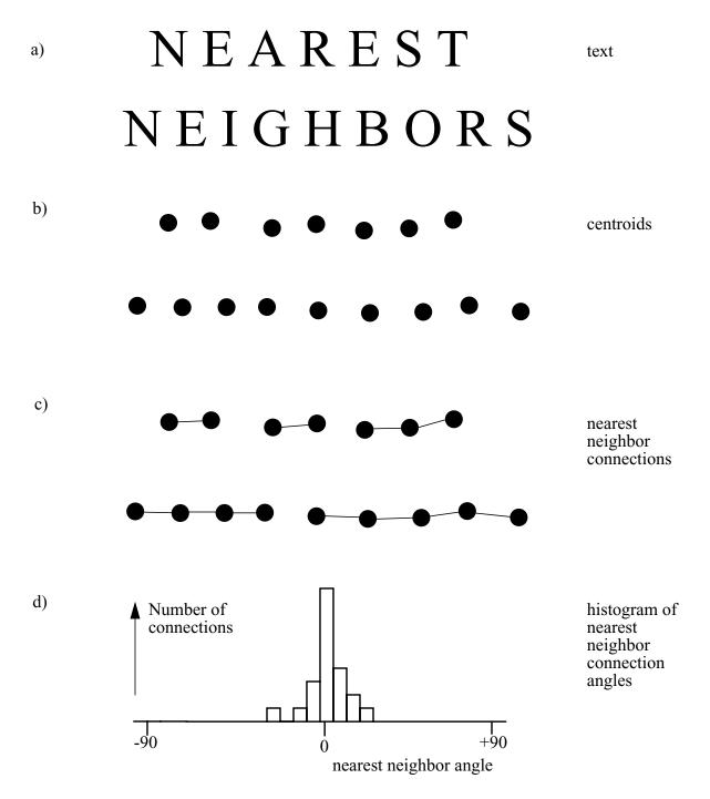
Figure 2. Diagram illustrates nearest-neighbor method. a) Text. b) Centroids of characters in (a). c) Connections between closest neighbors (1 neighbor each). d) Plot of connection angles showing peak at zero, indicating zero skew angle.
