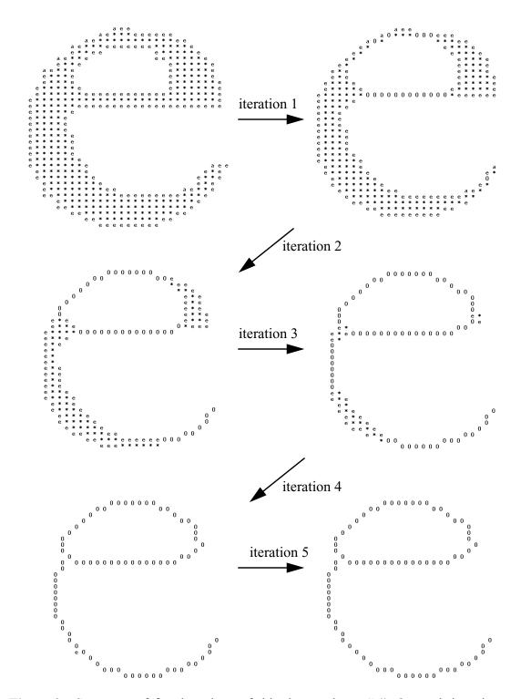
**Figure 2.** Sequence of five iterations of thinning on letter "e". On each iteration a layer of the outer boundaries is peeled off. On iteration 5, the end is detected because no pixels change.
