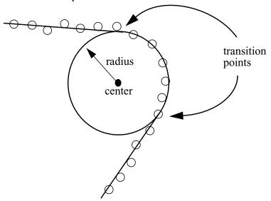
**Figure 2.** Circular curve fit to data points. Diagram shows parameters of this fit: two transition points from straight lines into the circular curve, and the radius and center location of the circle describing the curve.
