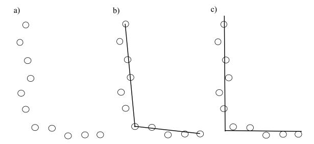
**Figure 1.** ON-valued pixels are shown in (a) and two corner fits are shown in (b) and (c). In (b), the fit is made exactly on data points. Because of this, the endpoints are sure to connect, but the corner angle is not as sharp as intended in the original. In (c), a least squares fit was performed to two sets of points, and the intersection of them was taken as the corner location. This yields a sharper corner.
