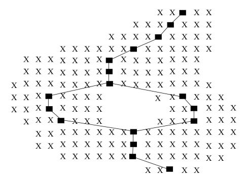
**Figure 2.** Line adjacency graph of region. The ON pixels are shown as "X"s. The middle of each row of ON pixels is shown as a filled box. The lines that join these midpoints of each ON row shows the line adja-
