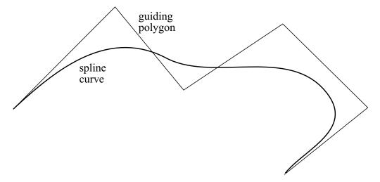
**Figure 3.** A spline curve is shown with its guiding polygon. The guiding polygon is from a straight-line polygonal fit to the image data. Notice that the spline lies within the corners of the polygon, thus yielding a smooth fit to the data.
