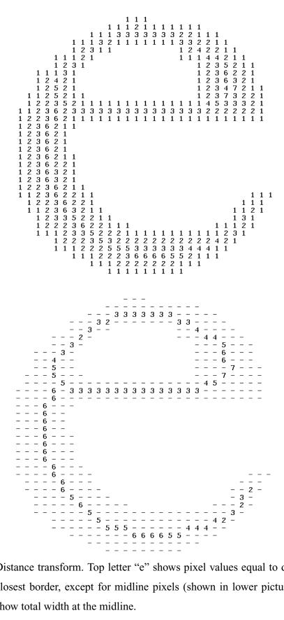
Figure 3. Distance transform. Top letter "e" shows pixel values equal to distance to closest border, except for midline pixels (shown in lower picture), which show total width at the midline.
