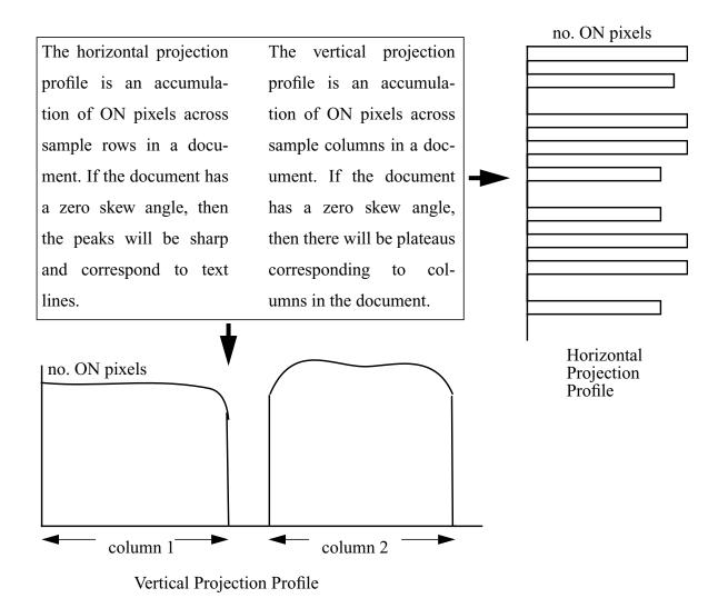
**Figure 1.** A portion of two columns of text are shown at the top left. The horizontal and vertical projection profiles from this text are also shown. Notice in the horizontal projection profile that each bin corresponds to a text line, and in the vertical projection profile, each plateau corresponds to a column.
