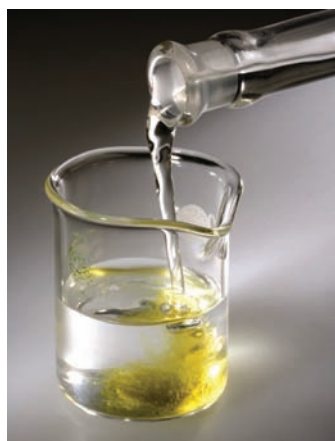
▲ Figure 1.5 Colourless chlorine water reacts with colourless potassium bromide solution to form yellow bromine.
