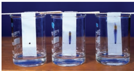
▲ Figure 1.8 Substances separate as they move up the paper with the solvent at different speeds.
