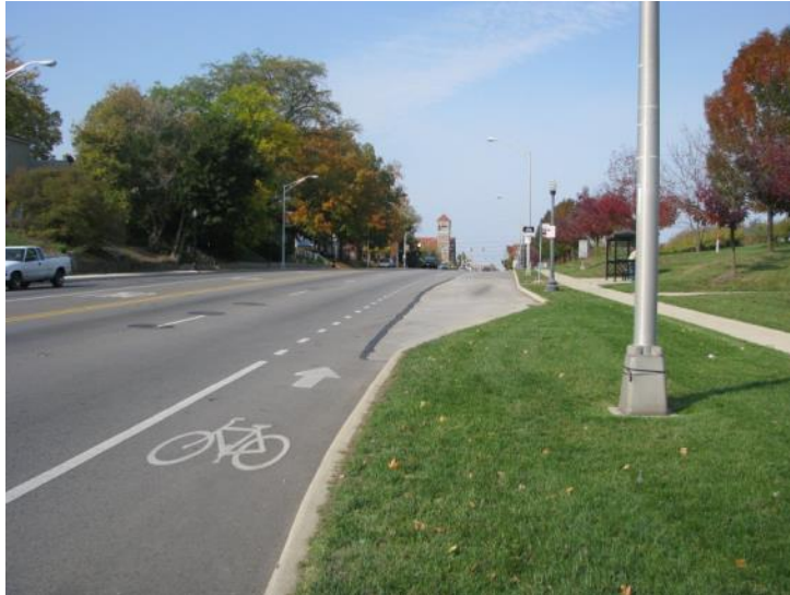
Figure 6-12 Bike Lane Dotting at Bus Stop Zone
