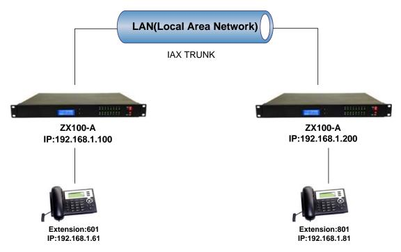
Register the ZX100-A as an peer in ZX100-B(via IAX2 trunk),so the extensions in ZX100-A can make calls to ZX100-B's extensions via this "special" trunk.
