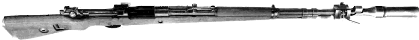
A WARTIME OPPONENT OF THE LEE-ENFIELD A German 7-92 SERVICE RIFLE fitted with Grenade Thrower.
