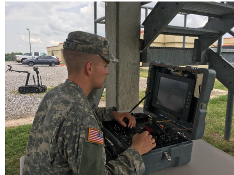
Cadet Middleton remotely operates a robotic arm (seen in background) that is used by Army EOD to safely dismantle explosive threats
