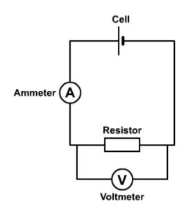
An ammeter needs to measure the flow of charge, so it is in **series**. This means that all the charge has to flow through it and can be counted. It also means that an ammeter needs to have a very low resistance.
