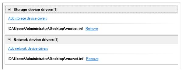
Recovery Media Builder can build 32-bit WinPE media configured to the uEFI mode, which is the only type compatible with Windows pads running on Intel Atom.
