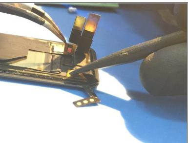
• I used a solder iron tip that was larger than the solder pads. Turn your soldering iron up to a high temperature, 350C is where I kept mine at. DO NOT add any solder, just use the heat & tweezers to pull back the tabs. After unsoldering pull the flex cable out of the way and use tweezers to peel back the proximity sensor from the AMOLED. CAREFULLY.
