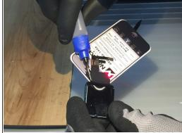
Begin by preheating the entire screen to a uniform temp, letting it sit under warm air for 10 minutes. I keep my heat gun on 300F-350F while holding the screen 3"-6" away from the nozzle to vary the temperature. Carefully insert a business card under the screen on the dig flex side. Use alcohol to weaken the OCA tape bond then move the card in slow
