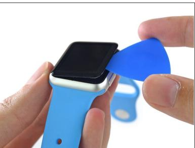
Heat the screen up so that the entire display and watch are warm. Be sure to turn the device off first by holding down the crown then sliding to power off. Using a sharp blade start at the bottom right corner and lift the glass up enough to create a gap, once you have a large enough gap use a plastic tool to break the adhesive bond around the edges
