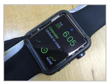
Be careful of the force touch flex cable that sticks into the frame on the bottom left of the display while removing the display assembly from the frame. The force touch gasket sits around the ENTIRE edge of the watch and is a thin silicone membrane. Test your AMOLED after separation before proceeding to the next steps.
