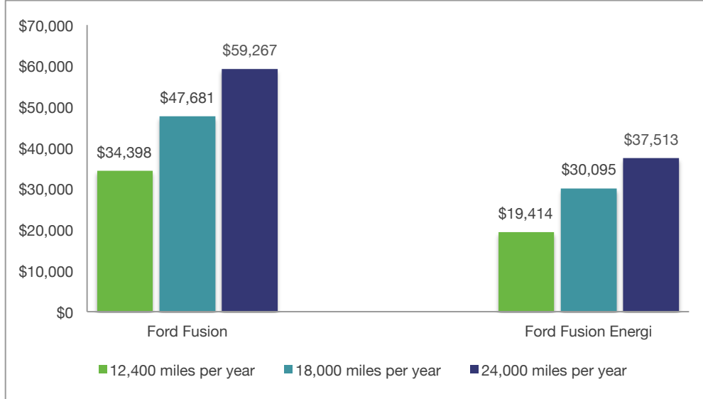
FIGURE 14: TOTAL COST OF OWNERSHIP OF CONVENTIONAL ICE VEHICLE VERSUS ELECTRIC VEHICLE BY ANNUAL MILEAGE
