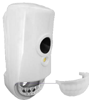
Figure 11: Insert the IPD Lens
