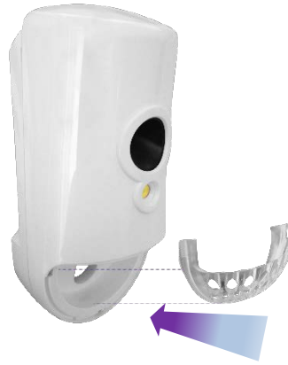
Figure 10 Insert Pet Immune Lens into the IPD
