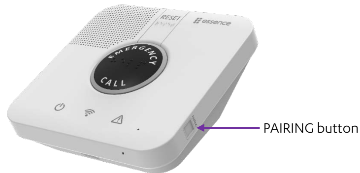
Figure 15: Press the CP PAIRING Button
