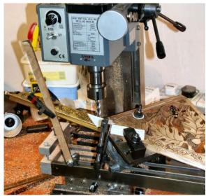
Fig. 6. Milling top of the knife edge where it intersects the polar gnomon. Note the stay supporting the gnomon tail.
