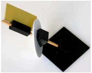
Figure 4 -- H2SS shadow plane and solar vane at sunrise on an equinox
