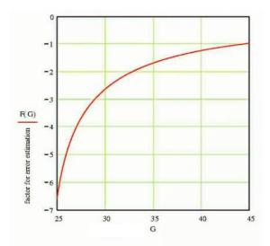
Fig. 2: Graphical representation of error estimation factor F from formula (19) depending on angle G; sun's declination  $\delta_S = 23.4393^\circ$ .
