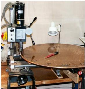
Fig. 7. Machining the edge of the dial plate, mounted on a motor-driven rotary table.
