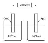
A student sets up a galvanic cell at 298 K that has an electrode of Ag(s) immersed in a 1.0 M solution of  $Ag^+(aq)$  and an electrode of Cr(s) immersed in a 1.0 M solution of  $Cr^{3+}(aq)$ , as shown in the diagram above.
