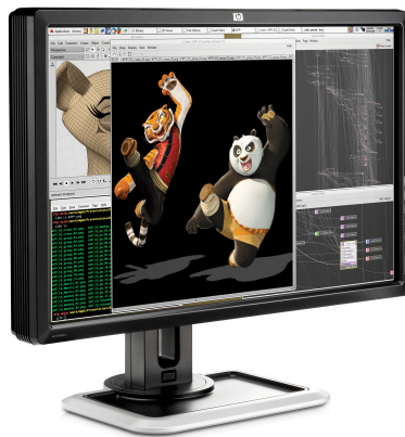
Figure 3: The HP DreamColor LP2480zx Professional LCD Display has a typical brightness of 250\text{cd}/\text{m}^2 and a typical contrast ratio of 1000 : 1. The BLU is a tri-color LED backlight and it covers 97% of the DCI-P3 gamut.
