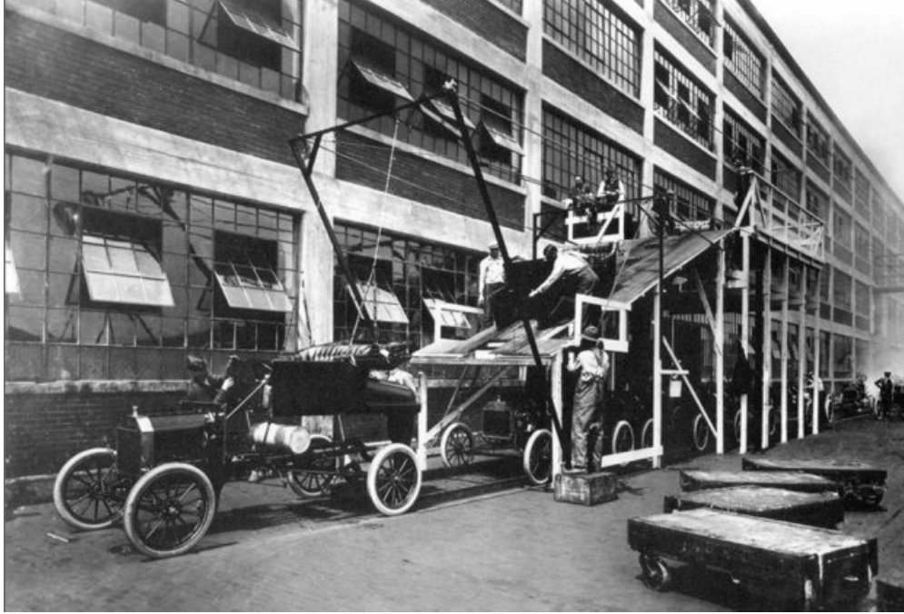
Model T assembly line at the Ford plant of Highland Park, Michigan circa 1913.
