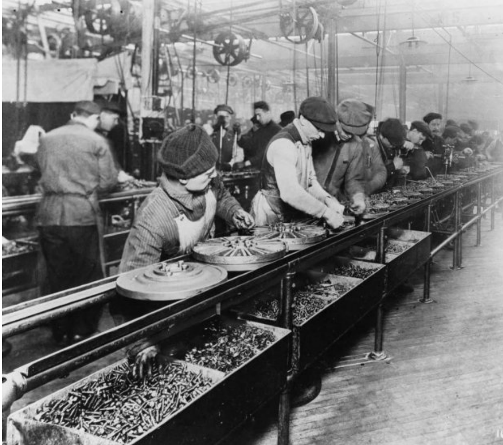
Highland Park plant assembly line fabricating magnetos and flywheels circa 1913.
