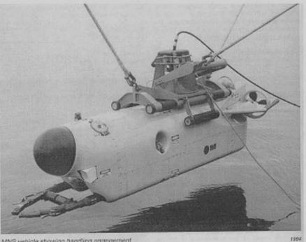
MNS vehicle showing handling arrangement
