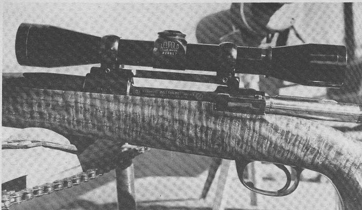
The six-power Leupold scope, held in place with Conetrol mounts, was fully stable and required little effort to bring to zero. (Left) Jack Lewis, for whom the custom rifle was built, checks it in his office.
