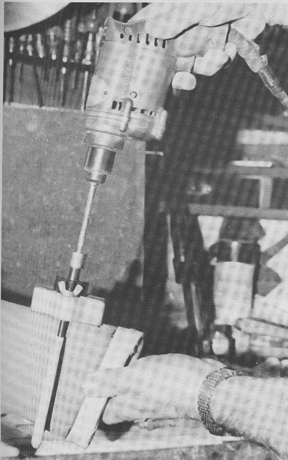
After stock has been sanded completely, the flush mount swivels are installed. Bish used a special jig for this.
