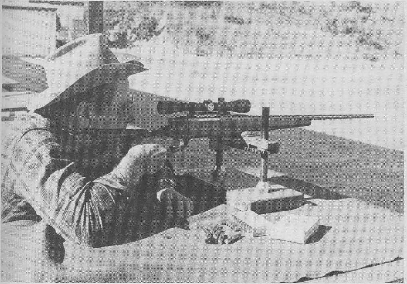
All of the test rounds were fired from a benchrest of special design. Recoil experienced with the thumbhole stock was found to be negligible, which is one claim that has been made for this stock design from its introduction.
