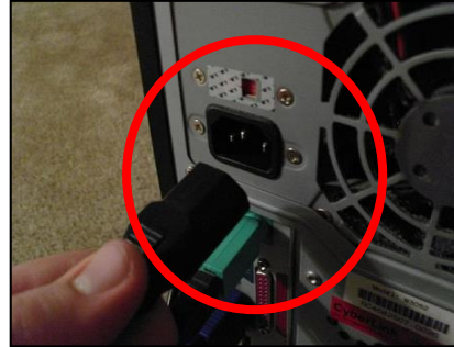
Figure 126. Unplugged Power Cable
