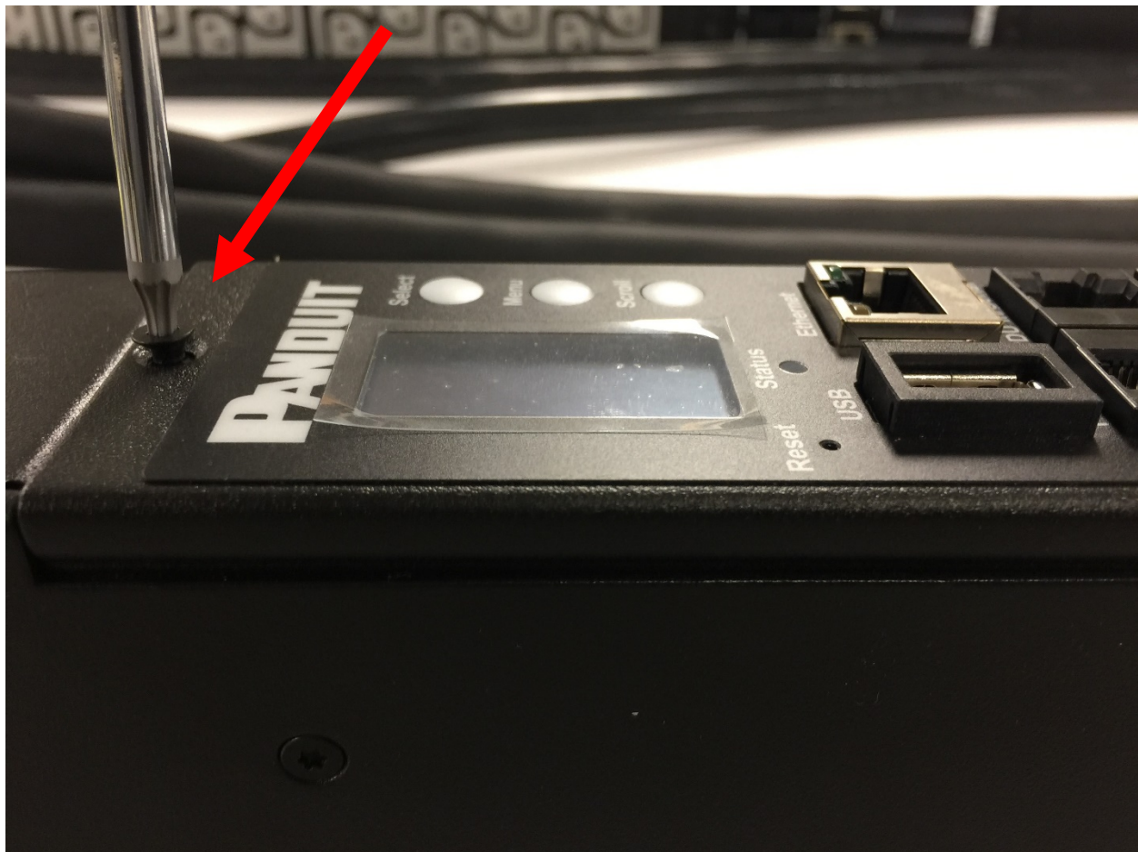
Figure 85: Removing Top and Bottom Screw from Intelligent Network Controller
