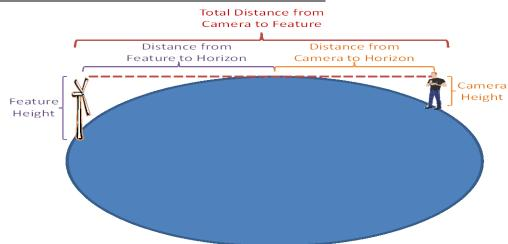
Distance from Camera to Horizon (miles) =  $1.312 \text{ x} \sqrt{\text{camera height (feet)}}$ Distance form Feature to Horizon (miles) =  $1.312 \text{ x} \sqrt{\text{feature height (feet)}}$
