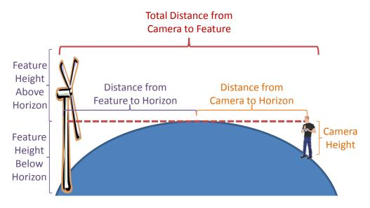
Next we need to determine how much will be below the horizon using: Feature Height Below Horizon (feet) = (Distance from Feature to Horizon (miles)  $\div 1.312$ )<sup>2</sup> = (6.79  $\div 1.312$ )<sup>2</sup> = 26.8 feet
