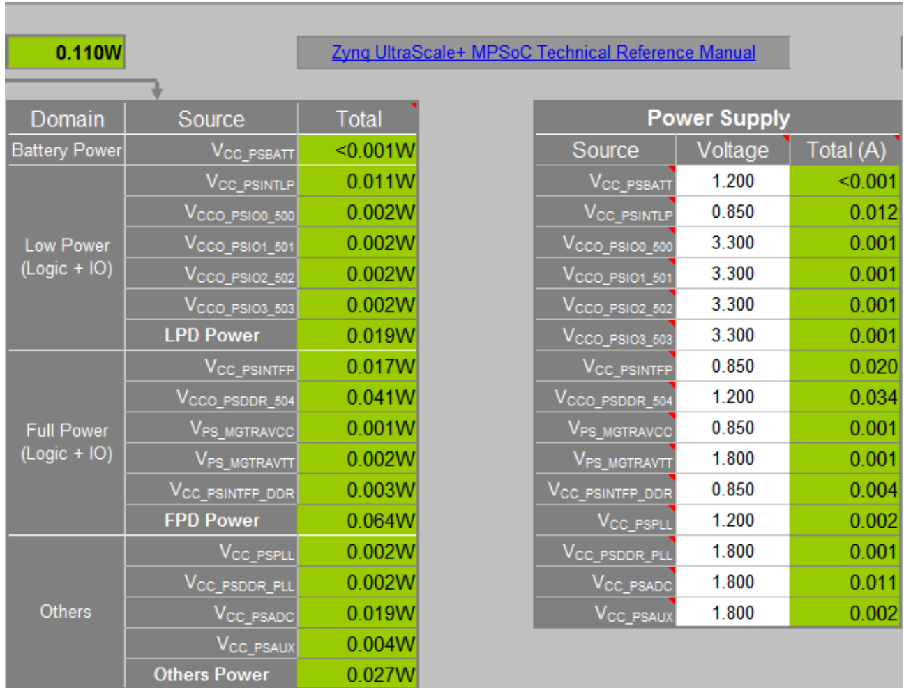
Figure 3-19: PS Sheet for Zynq UltraScale+ MPSoC displaying Sources and Power Supply
