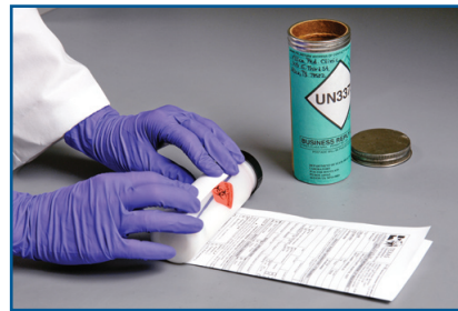
6. Place lab form around the outside of the liner. Place liner in cardboard mailer. Screw on appropriate, well fitting metal cap. Include return address and contact telephone number on label.
