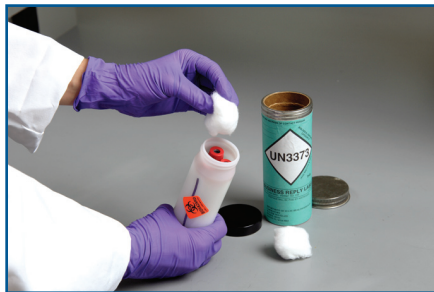
5. Place absorbent on top of tubes and screw on plastic liner cap.
